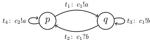
Figure 4: Example of a lossy channel system with two channels.
