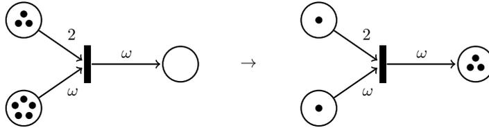
Figure 3: Left: example of an  $\omega$ -Petri net marked (counterclockwise) with  $(3, 5, 0)$ . Right: example of a possible marking, *i.e.*  $(1, 1, 3)$ , obtained after firing the unique transition.
